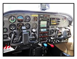
Image at left shows the older Cessna 206 cockpit configuration, and the image below shows new glass cockpit. The differences in cockpit equipment require additional training for pilots who operate these two configurations of aircraft and it requires additional flight hours to maintain proficiency. Not shown is the tactical radio equipment which provides encrypted air-to-ground communications.
