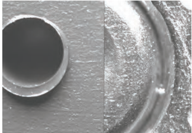
Figure 10: Gun 1, breech face cast (left) vs. breech face marks on fired cartridge case (right), 30X
