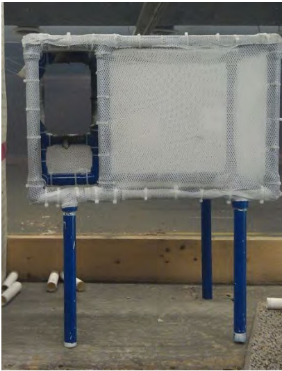
Figure 4. Brass catcher used to collect samples for this study.
