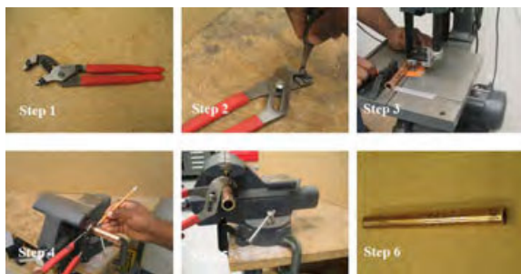
FIG. 10 Steps involved in the creation of tool marks from tongue and groove pliers.
